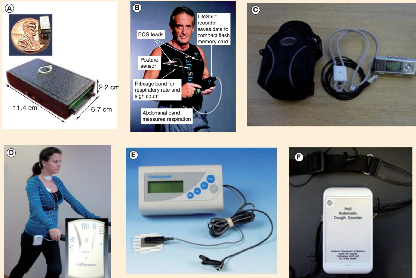
Figure 4. Objective cough monitoring devices. (A) Accelerometer Cough Monitoring (Penn State College of Medicine, PA, USA), (B) Lifeshirt™ (Vivometrics, San Diego, CA, USA), (C) Leicester Cough Monitor (Glenfield Hospital, Leicester, UK), (D) CoughCOUNT™ (Karmelsonix Ltd, Haifa, Israel), (E) Vitalojak (Vitalograph Ltd, UK) and (F) Hull Automatic Cough Counter (Castlefield Hospital, Hull, UK). Adapted with permission from [18].
