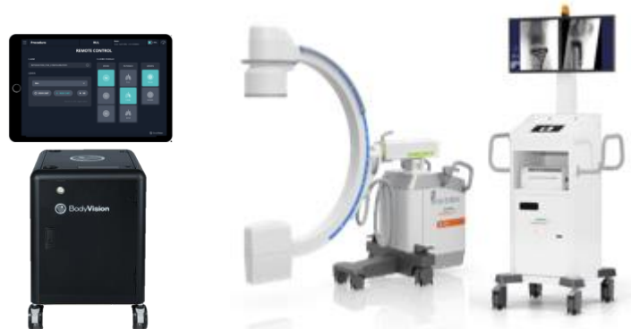
FIGURE 1. LungVision Platform. The platform integrates with available endobronchial modalities including bronchoscope, fluoroscope, and radial endobronchial ultrasound (REBUS) to present an augmented real-time pathway to a suspicious lung nodule. CT indicates computed tomography. ut
